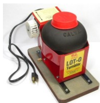
Vibratory type tumbler from the Rock Shed
